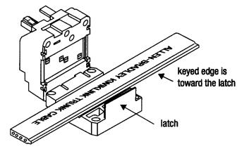
2. **Making sure that the cable is completely straight**, *carefully* close the hinged assembly, and apply firm, even pressure until the first latch locks into place.
